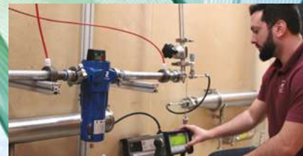
M-Plus Filtration's filter housings and elements performance has been tested to international standard ISO12500 series by IBR laboratory in U.S.A.
