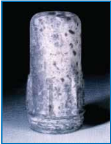
Rapid corrosion of untreated aluminium
